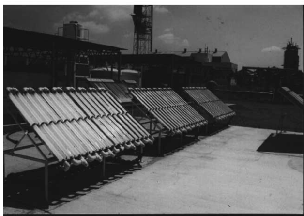
Fig. 1. Photo-reactors used at the Plataforma Solar de Almeria (Spain).
